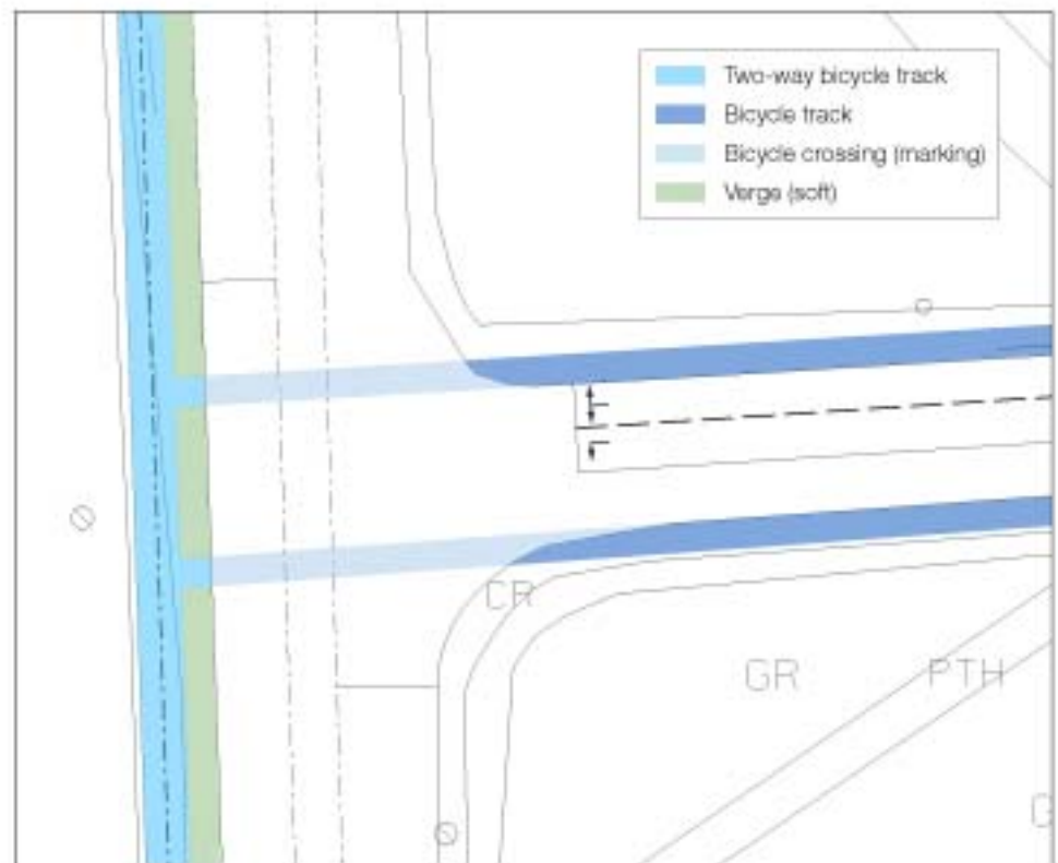
Figure 4.9 Proposed conceptual design for implementing bicycle facilities in the intersection Hanzas Iela/Eksporta Iela
