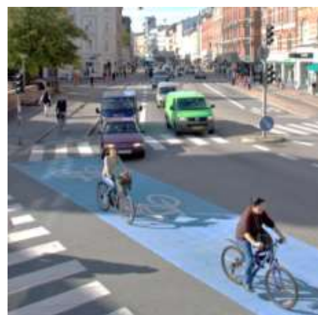
Figure 29 Intersection in Copenhagen with continuous cycling infrastructure through the intersection
